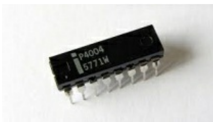
Intel 4004 Microprocessor Chip, 1971
